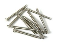
The Termination Technology range of electrical screws are fully threaded with a raised slotted countersunk head. Suitable for fixing face plates to a back box. The raised countersunk head is ideal for replacing screws that no longer reach the back box after plastering or tiling has sunk the back box further into the wall. Standardised thread size with a range of lengths available.
