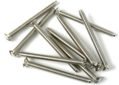
The Termination Technology range of electrical screws are fully threaded with a raised slotted countersunk head. Suitable for fixing face plates to a back box. The raised countersunk head is ideal for replacing screws that no longer reach the back box after plastering or tiling has sunk the back box further into the wall. Standardised thread size with a range of lengths available.
