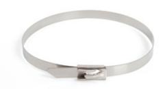
The Termination Technology TTSSBU range of bare Stainless Steel ties are manufactured from 316 grade material, offering a high corrosion resistance making them ideal for marine grade installation. Available from 150mm up to 1000mm lengths and in standard duty 4.8mm width, 7.8mm wide heavy duty available on request. TTSS 304 grade range also available with lower higher melting point but lower corrosion resistance, ideal for standard industrial applications.
