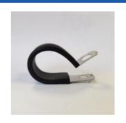
The Termination Technology range of rubber lined stainless steel p-clips are perfect for 18th edition compliant fixing of cable or conduit. Rubber lined to protect the cable or conduit from damaged caused by chafing. Available in a full range from 16mm-50mmØ.
