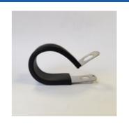
The Termination Technology range of rubber lined stainless steel p-clips are perfect for 18th edition compliant fixing of cable or conduit. Rubber lined to protect the cable or conduit from damaged caused by chafing. Available in a full range from 16mm-50mmØ.
