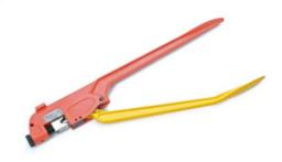
The Termination Technology TT95 indent crimp tool is designed for use with aluminium lugs from 10mm<sup>2</sup> to 120mm<sup>2</sup>. Hand operated with an adjustable jaw to set the tool to the correct size before crimping. Can be used for copper but designed for aluminium as it is a softer metal with a much thicker barrel which prevents the lug from splitting when crushing.
