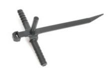
The Termination Technology wall plug cable ties are part of our specialist cable tie range. Manufactured in black with an integral wall plug and fixing pin designed to be a single part solution for fixing cables or small bundles to a wall. Supplied in a sealed pack with moisture absorbing silica gel to prevent them from going brittle. Manufactured from Nylon 6/6 offering high resistance to bases, oils, greases and chloride solvents.
