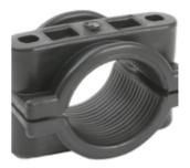
The Termination Technology range of nylon two bolt fixing nylon are a heavy duty method of fixing larger armoured cables where single bolt fixing would not be strong enough. Wrap the two halves around the cable and tighten the bolts to provide a tight and secure grip. Available in a full range to cover 41mm-105mmØ range, single bolt fixing cleats available for cables smaller than 41mmØ.
