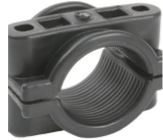
The Termination Technology range of nylon two bolt fixing nylon are a heavy duty method of fixing larger armoured cables where single bolt fixing would not be strong enough. Wrap the two halves around the cable and tighten the bolts to provide a tight and secure grip. Available in a full range to cover 41mm-105mmØ range, single bolt fixing cleats available for cables smaller than 41mmØ.
