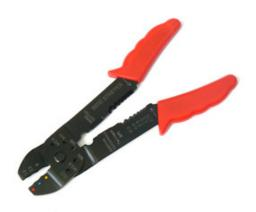
The Termination Technology SPI economy non-ratchet crimper is designed to be used with pre-insulated copper terminals. Hand operated with a separate jaw for red, blue and yellow terminals. Covering the full range of 0.5mm<sup>2</sup> to 6mm<sup>2</sup> insulated terminals. Wire stripper jaws for 0.5mm<sup>2</sup> to 6mm<sup>2</sup> above the handle to strip the insulation before fitting the terminals.
