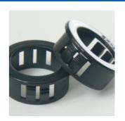
Nylon 66 snap fit bushes designed to turn sharp metal edged holes into smooth outlet holes, protecting cables and wires from snagging and being damaged. Suitable for use with junction boxes, distributor boxes, switch gear as well as any hole drilled with a hole saw. Supplied in trade counter packs of 25.
