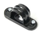
The Termination Technology range of fire-resistant spacer bar saddles are an efficient, 18th edition compliant way of fixing PVC conduits. Sizes available to fix 20 or 25mm diameter conduit in black or white. Prevents cable collapse in fire situations within commercial and industrial installations, fully ROSH and LSF compliant and Halogen free.
