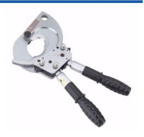
The Termination Technology range of ratchet cable cutting tools are used to cut cables in a variety of different sizes. Available in a standard range and an AR range which is suitable for cutting armoured cables. Using the standard cutting tools for armoured cables will quickly cause the cutting blades to blunt.
