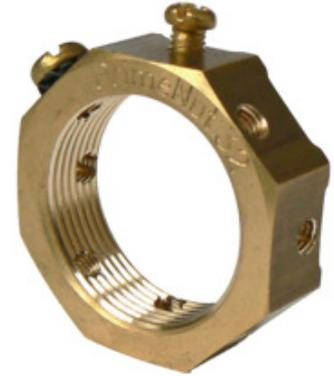
The Termination Technology range of brass earthing nuts revolutionise the installation of metal glands and enable a fast, easy and direct connection for protective earthing conductors. An earthing nut eliminates the possibility of loss of earth connection, especially where cables are terminated into a non metallic enclosure. Earthing nuts also provide a simple connection for both EMI/RF screening and protective earthing. Available in a range of M20, M25 and M32 sizes.
