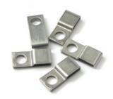
The Termination Technology P style stainless steel clip is an alternate way to fix cable ties. With a more flush style than the CTBSS which has a stand-off, they can be used in areas where there isn't as much space for the installation. Manufactured from 316 grade stainless steel and supplied in trade counter packs of 100.
