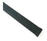
The Termination Technology range of expandable sleeving is made from heat stabilised polyester in either grey or black. The lightweight flexible screening provides a tough protection for bundles at temperatures up to +150°C. Available in a range of sizes and lengths in black and grey.
