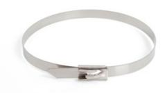
Our MET range of bare Stainless Steel ties are manufactured from 201 grade material, with a unique ball locking mechanism that allows for easy installation without coming undone. Available in common 200mm, 300mm and 360mm sizes with a width of 4.6mm.
