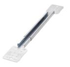
The Termination Technology range of pre-galvanized steel extendable mounting brackets are suitable for use in stud walls and floor joists, both wood and metal. Used for faster mounting of electrical boxes, conduit and pipework at multiple depths. Available in two sizes that cover a total range of 10"-24" (25-60cm) providing a quicker and easier method of installation compared to traditional methods.
