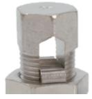
The Termination Technology range of Line Tap connectors are a form of mechanical connectors used to connect cable cores together. The split bolt allows multiple cables to be inserted and then tightened down onto a gripping plate to create a secure connection. These connectors are included and utilised in our branch resin joint kits to allow for the branch off connections.
