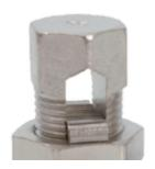
The Termination Technology range of Line Tap connectors are a form of mechanical connectors used to connect cable cores together. The split bolt allows multiple cables to be inserted and then tightened down onto a gripping plate to create a secure connection. These connectors are included and utilised in our branch resin joint kits to allow for the branch off connections.
