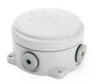
The Termination Technology of Industrial junction boxes are suitable for all surface applications. Manufactured from high impact, corrosion and UV resistant glass polyester. Provides 1, 2, 3 and 4 way versatility with multiple entries and a screw on lid, all providing an IP68 rating.
