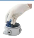
The Termination Technology range of Re-enterable gel is a bi-component rubber system insulating resin, designed for telecommunications and low voltage applications. Supplied as a two part pack with resin and hardener, breaking the seal will mix the two together and begin the setting reaction. Available in a range of pack sizes from 160ml up to 1650ml.
