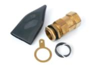
The Termination Technology range of EIFX ATEX rated brass glands are suitable for indoor and outdoor applications with SWA armoured cables and braided armoured cables such as SY, CY and YY. All packs supplied complete with glands, shrouds, brass locknuts and brass earth tags. Smaller sizes up to and including EIFX32PK are supplied in packs of 2, EIFX40PK and above are supplied in packs of 1.
