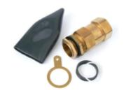
The Termination Technology range of EIFX ATEX rated brass glands are suitable for indoor and outdoor applications with SWA armoured cables and braided armoured cables such as SY, CY and YY. All packs supplied complete with glands, shrouds, brass locknuts and brass earth tags. Smaller sizes up to and including EIFX32PK are supplied in packs of 2, EIFX40PK and above are supplied in packs of 1.
