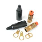
The Termination Technology range of EIFX ATEX rated brass glands are suitable for indoor and outdoor applications with SWA armoured cables and braided armoured cables such as SY, CY and YY. All packs supplied complete with glands, shrouds, brass locknuts and brass earth tags. Smaller sizes up to and including EIFX32PK are supplied in packs of 2, EIFX40PK and above are supplied in packs of 1.
