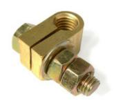
The Termination Technology EC range of earth clamps are used to connect single core cables to an earth rod. Keyhole style shape with a bolt intersecting, the cable lugs onto the bolt and as the bolt it tightened the clamp tightens onto the rod. Other styles such as our CS-EC rugby ball style are also available.
