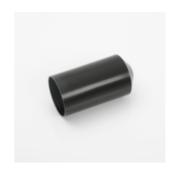
The Termination Technology range of Heatshrink end caps are manufactured from crosslinked polyolefin and internally coated with a hot melt adhesive to provide a watertight seal. Widely used to prevent contamination and moisture ingress of power cables during transportation and installation. Also offering excellent resistance to abrasion.
