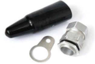
The Termination Technology range of aluminium armoured glands provide an IP66 rating and are suitable for both indoor and outdoor installation. Supplied in a kit of two in sizes up to and including M32 and kits of one in sizes M40 and above. All packs are supplied complete with glands, earth tags, lock nuts and PVC shrouds. A premium range is also available under the CW(size)ALP part codes.
