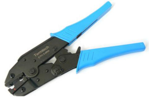
The Termination Technology range of ratchet crimpers include tools to crimp pre-insulated terminals, uninsulated terminals, bootlace ferrules and more. Single hand operation assisted by the ratchet. The range includes crush type crimpers, square section and hex section crimpers.
