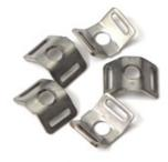
The Termination Technology stainless cable tie bases is an equivalent style to our CTBV nylon cable tie mounts. Manufactured in stainless steel, they are 18th edition compliant as they are a complete metal fixing. Two stand off wings protrude from the base allowing for a cable tie installation parallel to the wall. Manufactured from 316 grade stainless steel and supplied in trade counter packs of 100.
