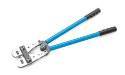
The Termination Technology heavy duty range of non-ratchet crimp tools are used to cover cables from 6mm<sup>2</sup> to 150mm<sup>2</sup>. Hand operated with rotating dies fixed in the head to avoid loose parts that can be lost. Dies are sized based on copper cables and lugs being used, for Aluminium jumping up a size or two can be an option as the material is much thicker.
