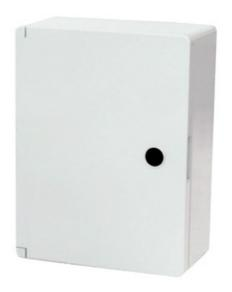
The Termination Technology range of IP65 Watertight Boards are available in a range of sizes to accommodate a wide range of applications. Manufactured from ABS in Grey (RAL 7035) with triangle lock-key. Supplied complete with a 1mm thick adjustable galvanized steel mounting plate and reversible door.
