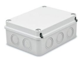
The Termination Technology wide range of junction boxes come in a variety of shapes, sizes, covers and fittings. All supplied in a light grey ABS material with high impact resistance. Metal mounting plates also available across the range. Sealing methods include stainless steel screws, 3/4 turn plastic encapsulated screws or press fit covers. Different methods offer different IP ratings. Hinged door plastic and metal enclosures are also available in a range of different sizes.
