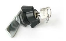
The Termination Technology range of key locks as suitable for use on our hinged door enclosures and watertight boards. Ideal for situations where the Allen key lock is not adequate and increased security is required. Available in two styles to suit our plastic and metal enclosures. To install, remove the hex key lock from the enclosure, thread the key lock in and screw together from the back.
