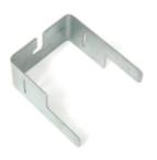
The Termination Technology range of trunking fire clips are an 18th edition compliant method of holding cables in place upon the trunking failing in a fire. Available in three different sizes to suit popular trunking dimensions and also available with a red coating for the 25mm trunking.
