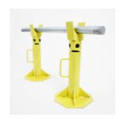
The Termination Technology range of cable jacks are suitable for lifting large drums of cable off the ground for easy reeling. Mechanical screw type operation with two jacks and a spindle bar. The Base plates on the jacks are designed to give stability even on soft ground. Available in 3 tonne, 6 tonne and 8 tonne versions.
