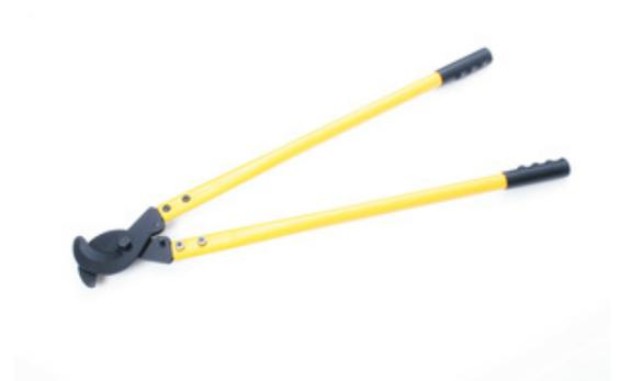
The Termination Technology range of heavy duty non-ratchet cutting tools are used to cut single core cables in a variety of different sizes. Hand operated with long and robust handles for optimal leverage and ease of use. Not suitable for armoured cables as this will quickly cause the cutting blades to blunt.
