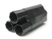
The Termination Technology range of Heatshrink Breakout Boots are available in 2 core, 3 core and 4 core arrangements and suitable for LV applications. Providing a watertight seal with the internal lining of low melt adhesive where cables enter connections or junction boxes.
