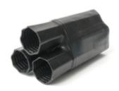
The Termination Technology range of Heatshrink Breakout Boots are available in 2 core, 3 core and 4 core arrangements and suitable for LV applications. Providing a watertight seal with the internal lining of low melt adhesive where cables enter connections or junction boxes.
