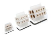
The Termination Technology range of insulated 4 way brass connectors are perfect for joining multiple cables in one connector block providing strong connections and insulation. Connector manufactured from brass to allow copper and aluminium connections to be made. Available in a full range to cover 1.5mm<sup>2</sup> to 120mm<sup>2</sup> cables, usable in our resin joint kits to provide extra insulation and a guarantee that the cores wont touch each other.
