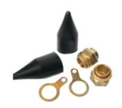
The Termination Technology range of BW LSF 2 Part brass cable glands suitable for steel wire armour (SWA) cable. Suitable for indoor application, all packs supplied complete with glands, LSF shrouds, Galv locknuts and brass earth tags. Smaller sizes up to and including BW32PK are supplied in packs of 2, BW40PK and above are supplied in packs of 1. CW LSF gland packs are also available as well as non-LSF in both ranges
