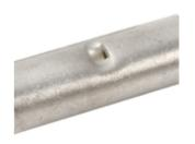
The Termination Technology range of copper tube butt splice connectors are designed for joining low voltage conductors. All connectors come with an internal taper at both ends for easier insertion of the conductors as well as a central stop to ensure correct core positioning before crimping. Mechanical connectors are also available from stock.
