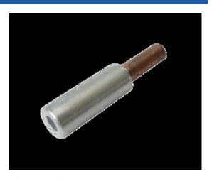
The Termination Technology range of Bi-Metal pins are suitable for terminating cables with aluminium conductors onto copper contacts without the risk of electrolytic corrosion and ensuring longevity. Supplied with a greased internal barrel and capped to prevent leakage. We would recommend using an indent crimper as aluminium is a softer metal than copper and the wall thickness of the lug is thicker to compensate.
