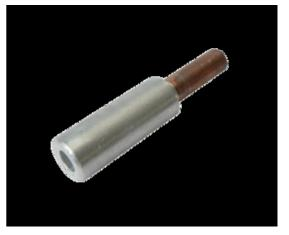
The Termination Technology range of Bi-Metal pins are suitable for terminating cables with aluminium conductors onto copper contacts without the risk of electrolytic corrosion and ensuring longevity. Supplied with a greased internal barrel and capped to prevent leakage. We would recommend using an indent crimper as aluminium is a softer metal than copper and the wall thickness of the lug is thicker to compensate.
