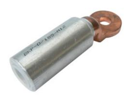
The Termination Technology range of Bi-Metal lugs are suitable for terminating cables with aluminium conductors onto copper busbars without the risk of electrolytic corrosion and ensuring longevity. Supplied with a greased internal barrel and capped to prevent leakage. We would recommend using an indent crimper as aluminium is a softer metal than copper and the wall thickness of the lug is thicker to compensate.
