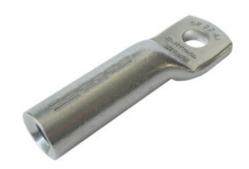
The Termination Technology range of standard aluminium tube terminals are suitable for termination cables with aluminium cores without the risk of electrolytic corrosion. Supplied with a chamfered entry for easy cable entry. We would recommend using an indent crimper as aluminium is a softer metal than copper and the wall thickness of the lug is thicker to compensate.
