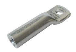
The Termination Technology range of standard aluminium tube terminals are suitable for termination cables with aluminium cores without the risk of electrolytic corrosion. Supplied with a chamfered entry for easy cable entry. We would recommend using an indent crimper as aluminium is a softer metal than copper and the wall thickness of the lug is thicker to compensate.
