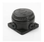
The Termination Technology range of explosion proof junction boxes are manufactured to be highly resistant to impact and ingress. Available in a smaller size with M20 entries and a larger with M25 entries, both with a screw down cover and ATEX rated for installation in hazardous areas. Also available in an industrial specification style using JB part codes.
