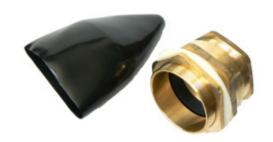
The Termination Technology range of A2 Brass cable glands are suitable for use with all types of unarmoured cable. Suitable for indoor or outdoor use by producing a weather proof seal on the outside of the cable. Supplied in complete packs with gland, locknut and PVC shroud. Sizes up to and including M32 come as packs of 2, M40 and above as packs of 1.
