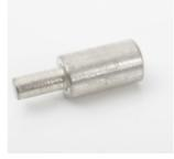
The Termination Technology range of bare Solid Reducing Pins are designed to reduce down conductor size when cables are oversized for control gear and MCB's. The pin makes these terminals ideal for terminating conductors into contact blocks. The range covers sizes from 10mm<sup>2</sup> to 400mm<sup>2</sup> with larger sizes up to 1000mm<sup>2</sup> being custom made to request.
